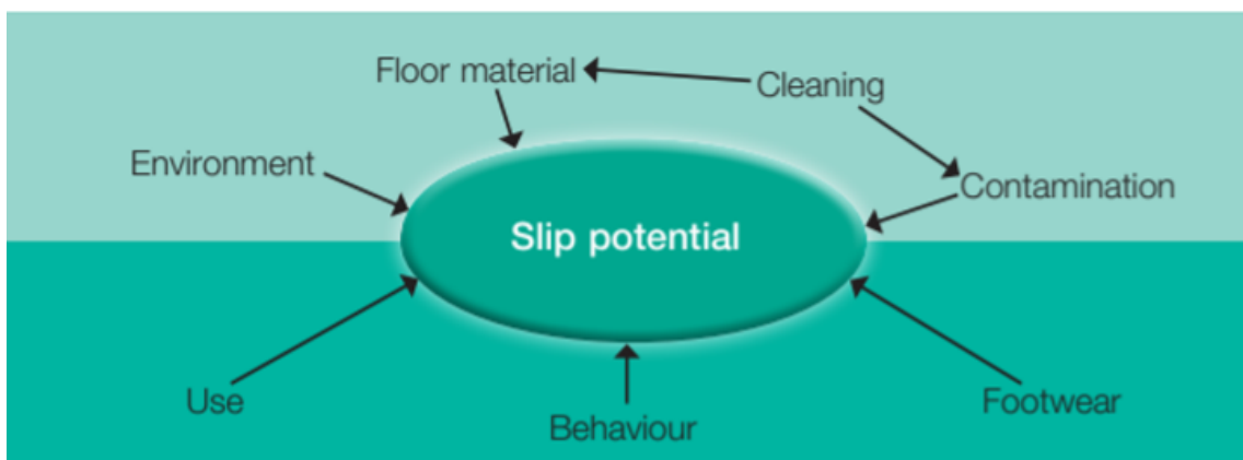
Slip potential model from HSE Technical Information Sheet 'Assessing the slip resistance of flooring'
