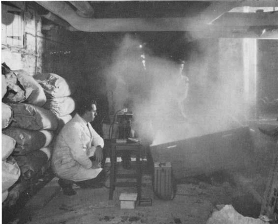
Fig 4: Air sampling by thermal precipitator during mixing of magnesia/asbestos plaster with water
